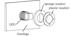
Caution: Plastic washer should be pressed with an even force all around the surface of washer, or it can break.
